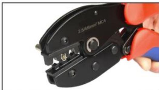
Paso 3. Inserte el conector MC4 en la ranura adecuada (2.5/4.0/6.0 mm<sup>2</sup>)
